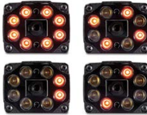
Independent lighting controls
