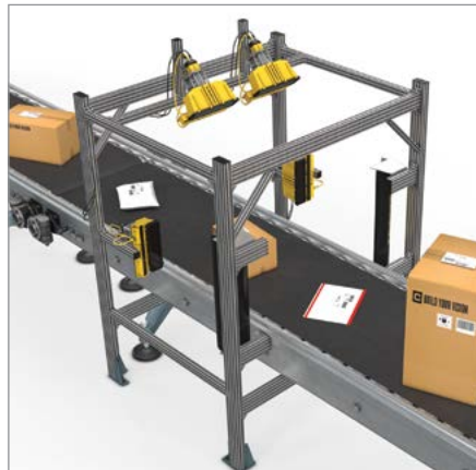
Multi-sided scan tunnel
